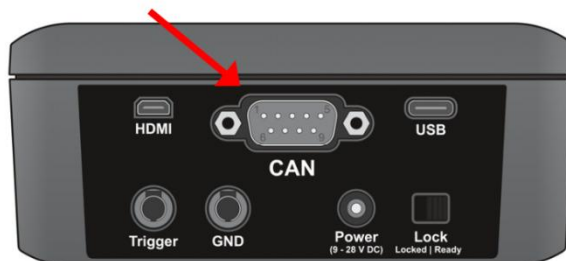
CAN connector (D-Sub) on the rear of the device
